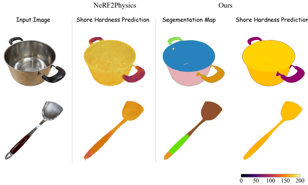
Figure 11. Qualitative comparison of hardness prediction. Compared to NeRF2Physics, our method provides more accurate hardness prediction with clear boundaries.
