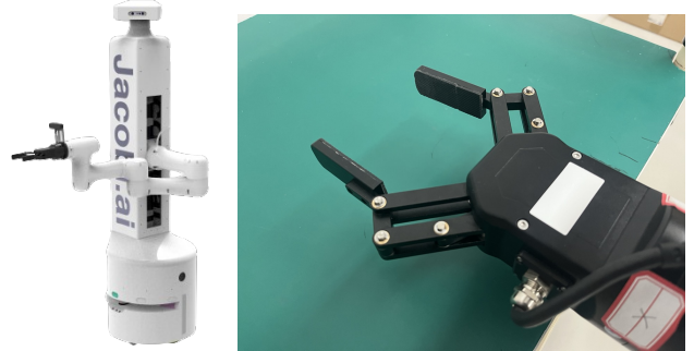
Figure 7. The robot platform (left) and the robotic gripper (right) utilized in robot grasping experiments.
